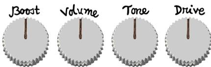
**BOOST:** Sets the boost level, which is engaged with the left stomp switch. [Start around 11:00 o'clock]. The Drive and Boost controls are based on my original Super Hard On™ gain control, so they may crackle when turned. This is perfectly normal.
