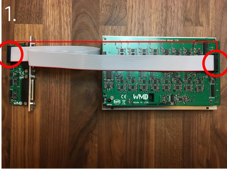
1. First, connect the far-right 20 pin connector on the Performance Mixer to the 20 pin header on the very top of the DB25 expander with the included 20 pin ribbon cable.
