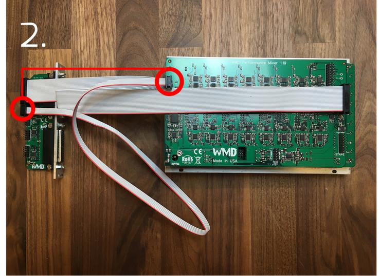
2. Next, connect the top-most, far-left 6 pin header on the PM to the 6 pin header on the DB25 expander directly below with the included 6 pin ribbon cable.
