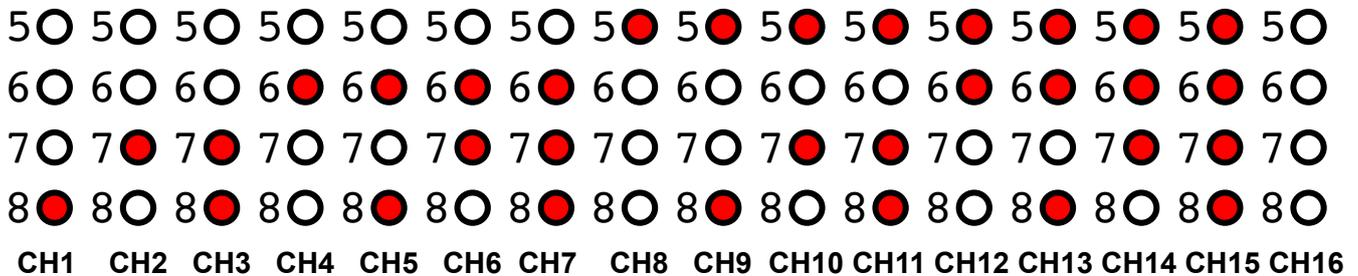
**MIDI note page:** use ↑ and ↓ to select MIDI note for the **last active trigger**, hold ↑ or ↓ to save and exit, LEDs flash fast. LEDs 5-8 will display the last 4 bits of the note number in binary
