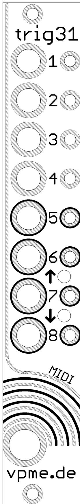
**Basic operation:** connect trigger or gate signals to inputs 1-8, connect **MIDI-out** to MIDI device
