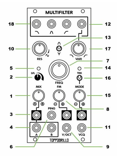
1- MIX knob 9- V/OCT CV input 17- MODE select control
