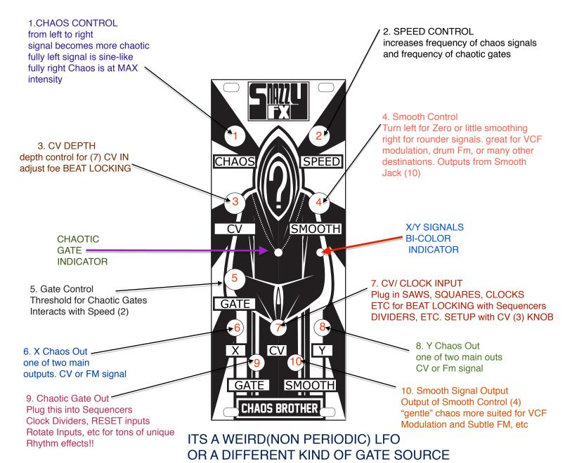
USE X/Y outs with X/Y mode on a scope /phase meter to watch the attractor!
