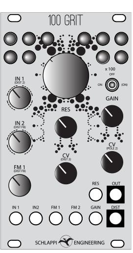
**TOUCH POINTS** 8 brass balls connected to sensitive points in the circuit and voltage control points. Touch more than one at a time or use with conductive materials as resistive patch points.
