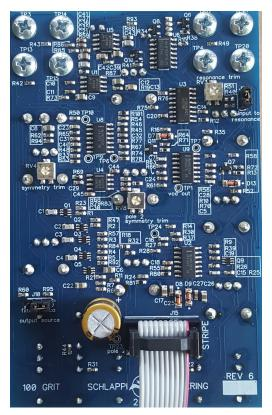
Please ensure that the red stripe is aligned to the -12V rail on the eurorack case power as well.
