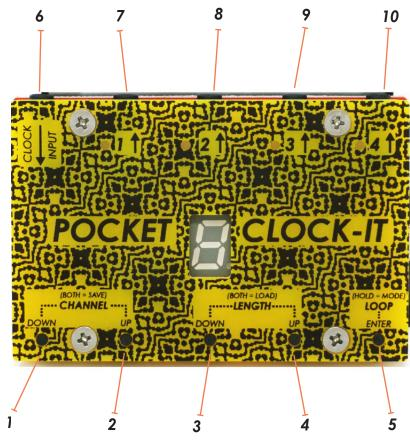
HOW TO SWITCH MODES: Hold LOOP / ENTER button to switch modes. When a lower case "r" is displayed, POCKET CLOCK-IT is in random mode. When an upper case "C" is display, POCKET CLOCK-IT is in clock divider mode.
