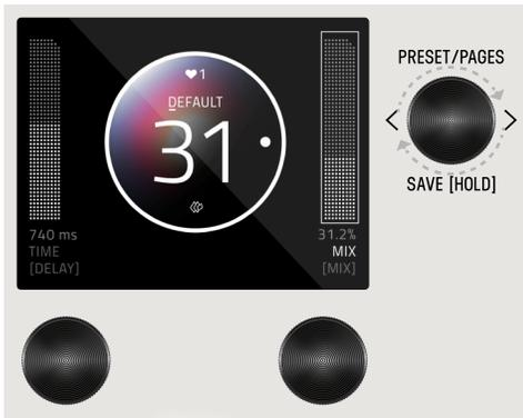
In the [EDIT PAGE](#), if a parameter was assigned as a FAVORITE PARAMETER, a filled in L or R dot will appear to remind which side it was assigned. Favorite parameters can also be quickly assigned to **C1** or **C2** in the EDIT PAGE. Simply hold **C1** to assign the current parameter to **C1** or hold **C2** to assign the current parameter to **C2**.
