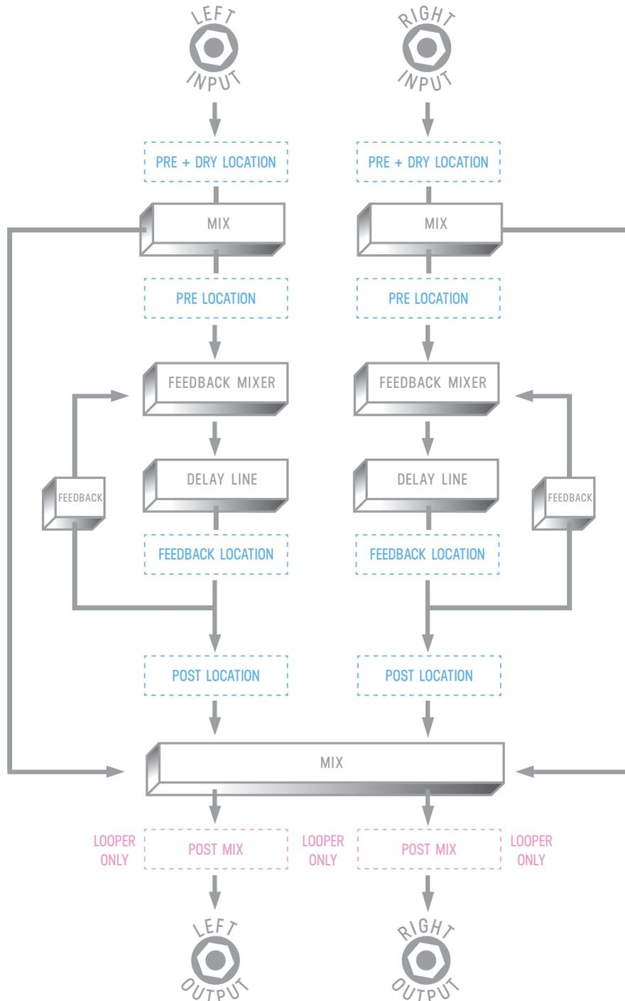
Also shown in the visual diagram is the Mixer for LVX. The Mixer is directly connected to the front panel mix knob. To adjust the Dry and Wet Trim levels, use **C3** to enter Edit View and page over to the MIX section. The following is a breakdown of each Category and the processing Elements they contain:
