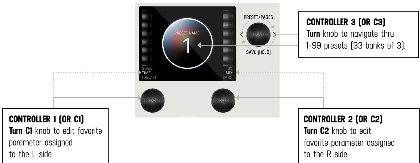
**NOTE:** GRAPHIC VIEW is designed to focus on 1 block and/or 1 parameter at a time per preset. [You have the option to switch to "[TEXT VIEW](#)" in GLOBALS -> EDIT PAGE. Favorite Parameters are also available in [TEXT VIEW](#).
