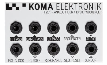
The patch bay consists of ten 1/4" mono jack sockets which you can use for receiving and sending various audio or control voltage signals. Blank arrows mark CV inputs/outputs, black arrows mark audio inputs/outputs. If the arrow is pointing towards the jack socket it shows you that this is an output, if the arrow is pointing away from the jack socket it is an input.
