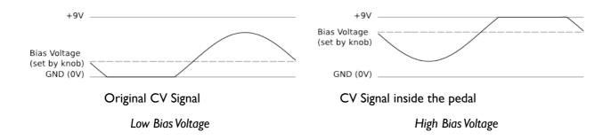
A similar thing happens to unipolar CV signals: Their point of origin (0V) is shifted by the amount set with the corresponding knob. In other words: You add the voltage of your knob to the voltage of your incoming unipolar CV signal.
