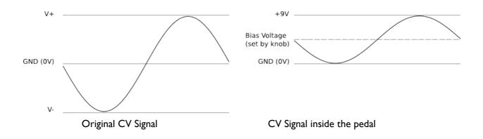
So, what happens? The incoming CV signal is shifted around the voltage that you select with the corresponding knob. Example: if you insert a -5V to +5V sine wave into the RESONANCE CV jack you will
