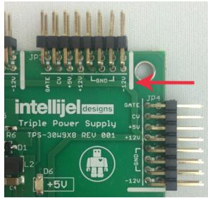
Once connected, the cabling between the module and power supply should resemble the picture below:
