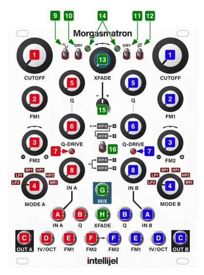
controls how deeply the cutoff frequency is modulated by the signal appearing at FM1.
