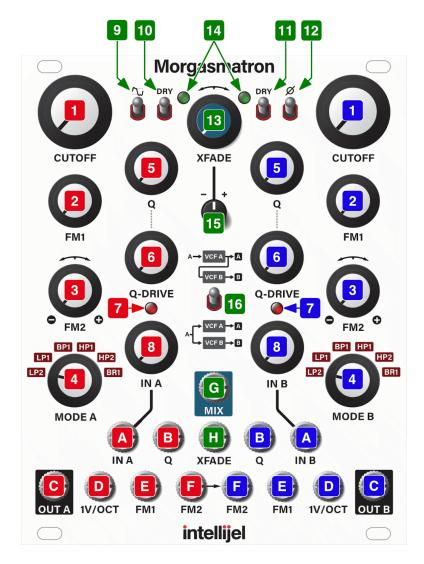
Once you bypass a filter using its DRY switch, you can use the XFADE knob (in conjunction with the MIX out) to set a wet/dry mix between the processed and unprocessed signals. For example, if you turn on the OVERDRIVE circuit for Filter A and set Filter B to DRY, the XFADE knob acts a wet/dry control for distortion.
