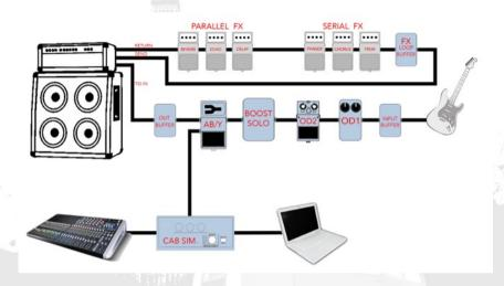
As in the sample rig below, you can use your 1959DD both in front of amp and, via the D.l.out, to mixer or DAW simultaneously for a nice live monitoring or excellent quality live recordings.
