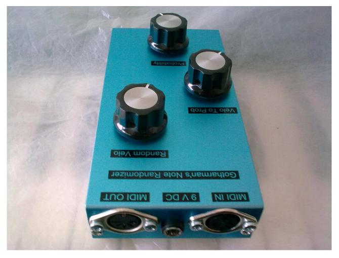
**MIDI IN:** Connect this to MIDI out from a MIDI device like a keyboard or a sequencer, that transmits MIDI note on's and off's.
