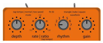
Plug your guitar into the jack on the right side. Plug your amplifier into the jack on the left side. Set the mode switch to "tap tempo" and set the waveform switch to "tube". Set depth to half, rate to 1:2, rhythm to 1 (all the way counterclockwise), and gain to one half. Now tap the tempo you would like using the tap stomp switch.
