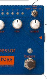
**meter:** red LEDs indicate gain reduction (gr). Gain reduction values are marked over each LED.
