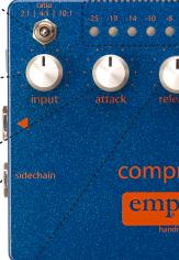
**release:** controls how quickly the compressor retuns to its initial level. Release time increases as your turn the knob clockwise. **Range:** 50ms - 1s
