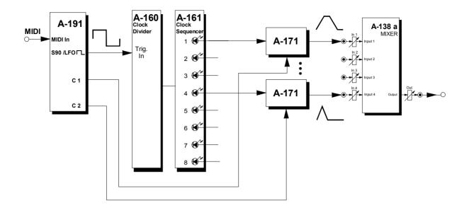
Fig. 5: Producing complex controllable modulations.
