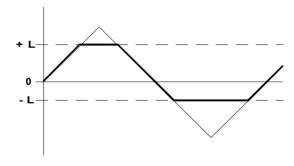
**Fig. 1**: how the clipping levels work (input signal = triangle)
