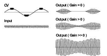
**Fig. 2**: Resulting amplification with bipolar control voltage (CV) and different gain settings
