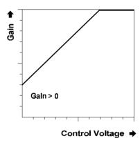
Fig. 1: Effect of gain control on VCA response
