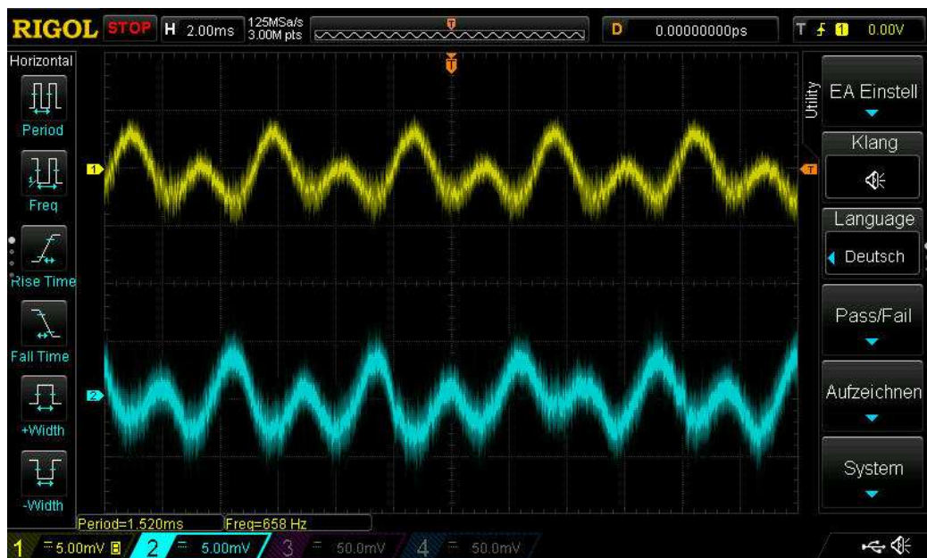
Typical Oscilloscope picture for ideal adjustment of RM1 and RM2 (5 mV / grid)
