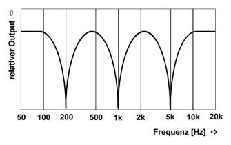
Fig. 1: The principle of phasing
