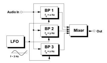
Fig. 2: A phaser model using separate modules
