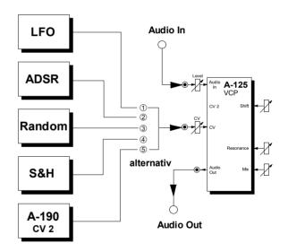
Fig. 3: Typical phaser application
