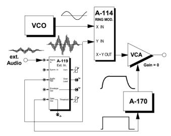
Fig. 3: Ring modulator squelch patch
