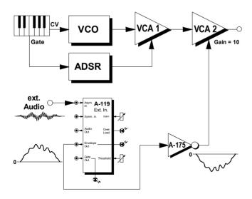
Fig. 4: "Ducking" by using an external signal
