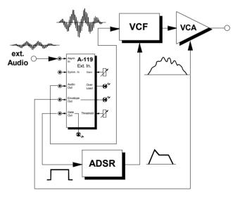
Fig. 2: Filtering an external audio signal
