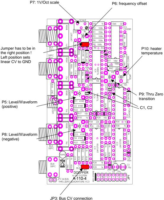
when installed the bus CV is connected to the switching contact of the 1V/Oct socket
