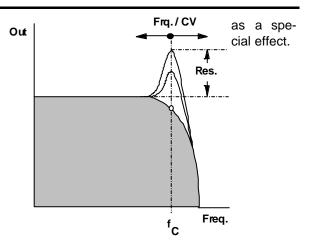
Fig. 1: Frequency response of the A-103
