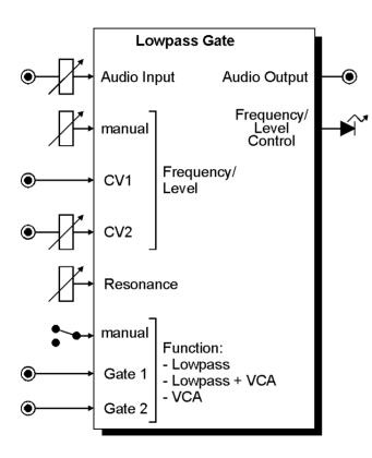
Module A-101-2 is a vactrol based combination of Low Pass filter (LP) and VCA. Additionally a combined mode LP+VCA is available. In this mode the sound becomes more dull as the loudness decreases. The A-101-2 was inspired by module 292 of Don Buchla. He also intruduced the term "Low Pass Gate" for this combination of functions.
