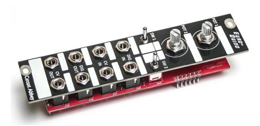
Now invert the assembly and start soldering. Make sure all the components are pressed down all the way, especially the switches.
