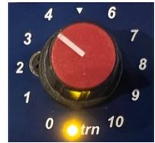
Try it! The yellow LED will flash with every octave shift and you should hear the results. (CV changes out the “pitch” banana don’t occur until position 3.6. See the chart below.)
