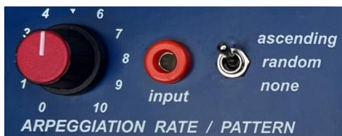
To the right of portamento is the **Arpeggiator**. The 218 will arpeggiate based on the keys that are sustained with the fingers or sustain pedal. The switch determines the **PATTERN**: whether the arpeggiation is active or whether it plays an ascending or a random pattern. (For more random options, see the appendix for information on how set and play with “directed random”).
