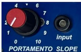
To the right of these outputs is **Portamento** control. Adding portamento will make the pitches slide from one to the next like a violinist sliding a finger to the next pitch. It is an endearing musical affect. To control the speed of the slide, turn the knob higher. At 0, it does not slide; At 10 it may take several seconds to reach the next pitch. The input banana is another way to control this parameter with a CV. The CV input will add to the portamento time set by the knob.
