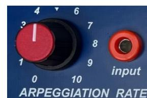
Easiest: Keep the Arp pulse input and reassign the portamento CV input to the Arpeggiation rate with a firmware change: If you don't use the portamento CV input, you can reassign that hardware input to control the Arpeggiation Rate. Look on the website for the Firmware that is listed as with "Porta\_CV\_to\_Arp\_Rate" in the titled like 218eV3\_v362\_Porta\_CV\_to\_Arp\_Rate\_DFU.hex and follow the firmware update instructions.
