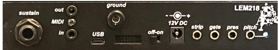
**Sustain:** The Easel comes with a ¼” connection labeled “sus” or “sustain.” The keyboard will hold one pitch or latch arpeggiated pitches while holding down sustain. In Polyphonic MIDI mode it will transmit MIDI CC64 unless it is in an arpeggiation setting. The pedal holds notes in mono mode, but does not send MIDI CC64. You can use either normally-open or normally-closed pedals. The polarity of your sustain pedal will be sensed on power up or during a reset button press.
