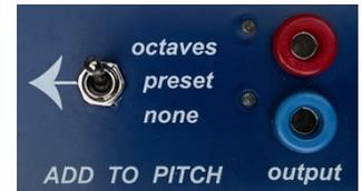
In monophonic mode the transposition will imitate the instant transposition of the pitch CV output and – if you are holding a key with a finger or sustain pedal – will play a new MIDI note when you touch the pad.
