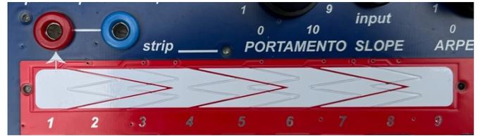
Try it out! The blue banana output is a 0-10v output range. Two blue LEDs at the ends help to indicate when the voltage approaches 0v or 10v, and the middle LED indicates the overall voltage level. The LEDs are directly controlled by the CV output.
