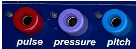
The **pulse** output is red banana on the upper left. A red LED will indicate every pulse output. The **pressure CV** output correlates to the detected amount of finger contact on the current/last single key touched. The blue LEDs next to the pressure output will get brighter as the voltage gets higher.
