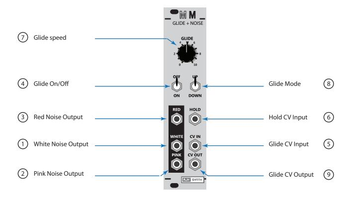
1) White Noise Out: This is the White Noise Output and signal level is +/-5 Volts peak to peak. Pure white noise is a sound that contains every frequency within the audio range (generally from 20 hertz to 20 kHz) in equal amounts. This white noise is generated by using a specially selected transistor in avalanche mode and using the exact circuitry from the Model D synthesiser, so it is a vintage analogue approximation of pure white noise.
