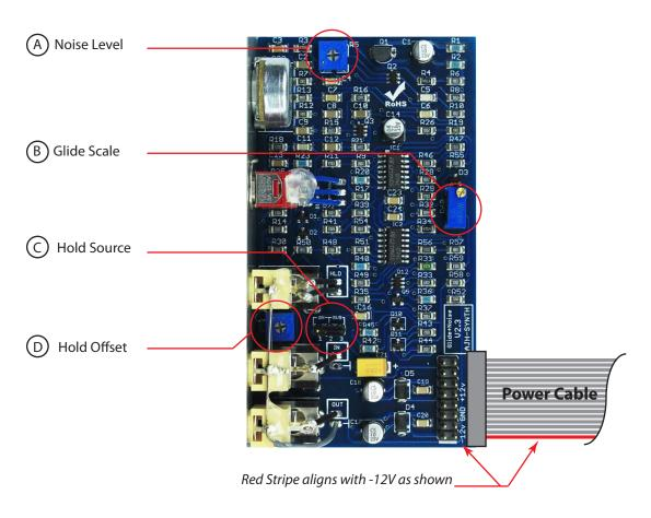
(A) Noise level: Sets the output level of the White, Pink and Red Noise. This should be set to +/- 5 Volts
