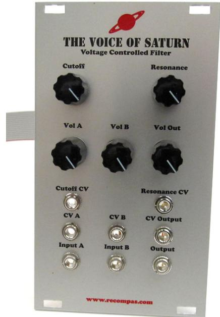
**Cutoff CV (0-5V):** Input control for the cutoff frequency of the filter
