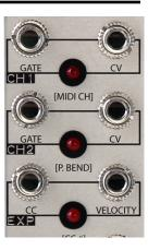
**Channel 1 Gate Out -** Channel 1 gate outputs a signal of either 0v (off) or 5v (on). This signal can be used to trigger an envelope generator, sequencer, logic module, or any other module that requires a gate input. The Channel 1 Gate is active when the Channel 1 LED is lit.
