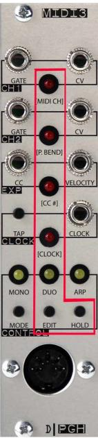
**EDIT MIDI CHANNEL** - The MIDI CH parameter assigns the midi channel. Pressing the HOLD button cycles through available options. Respond to all channels followed by channel 1 through channel 16. The number of times the LED blinks corresponds to the selected midi channel: 1 blink for channel 1, 2 for channel 2, etc... For all channels, the LED will blink at a steady rate.
