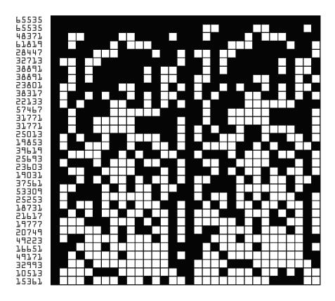
Variatic Erumption's patterns are based off of the bit-reversed concatenation of two 16-bit prime numbers. Prime numbers are always odd so in binary the lowest bit is always set. Reversing these will always generate a pattern who's first beat is set. Note the first two patterns are not prime as they are all bits set since this is the most simple burst pattern.
