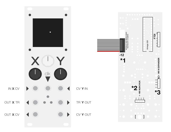
The CV Graphic is built around an Atmega328 chip, an 128.128 OLED screen and two DAC. The main idea behind the module is to provide interraction between CVs and Graphics, where graphics become a virtual partner in the musical creative process.
