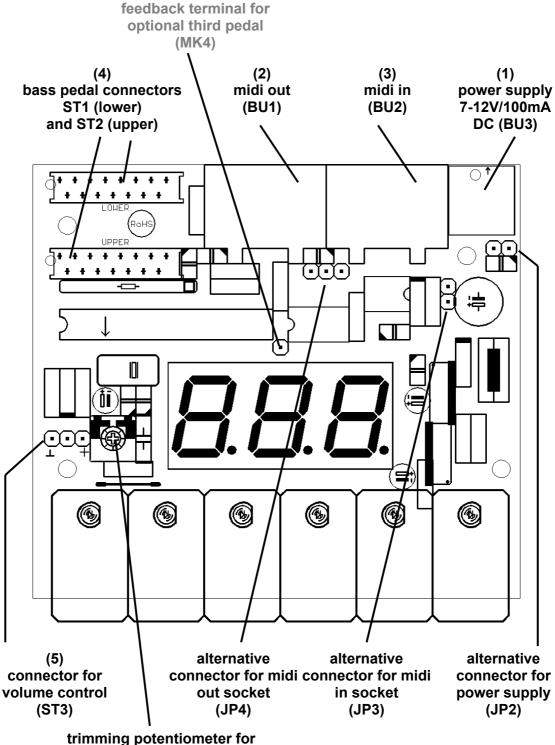
trimming potentiometer for voltage range adjustment of the volume control connected to ST3
