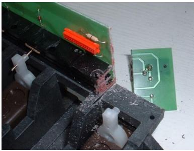
View after the pc board and the black plastic bar are cut off
