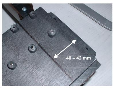
Mark a cutting line with a distance of about 40-42 mm from the edge to the bottom of the pedal frame.
