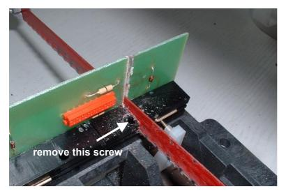
Cut also the black plastic bar which holds the pedal contacts with a suitable saw.
