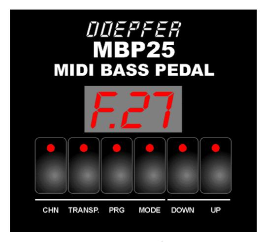
The three-digit display is used to show the value of the currently selected parameter, i.e. midi channel, transpose, program change number or mode. The LEDs indicate the currently selected menu.
