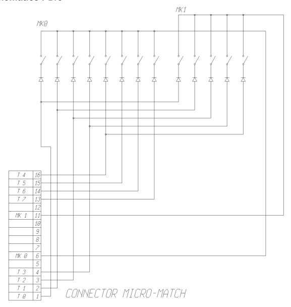
If another bass pedal or single contacts/switches are connected to the MBP25 they have to be wired identically to the PD/3.
