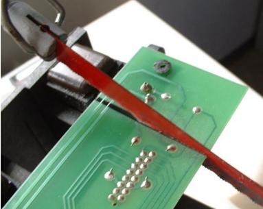
Mark a cutting line with a distance of about 32-34 mm from the pcb edge to the bottom of the pcb.
