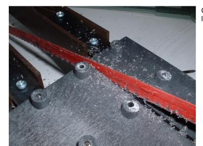
Cut off the pedal frame at this line with a suitable saw.
